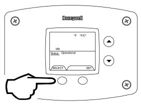
Step 2: Press "Set" button to change temperature format. "°F/°C" symbol will flash in the water heater display.
